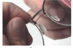
Align the two bridges, so that the rim's bridge is in the front of the bar's bridge.
