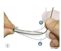
Fix the plane of the lens. Maintain it, adjusting the tilt of the temple with reference to the support point (ear) by means of large movements that exceed the elastic limit. The lateral grip point must be on the end piece of the bar, not on the temple.
